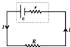
For a freshly prepared cell, the value of internal resistance is generally low and goes on increasing as the cell is put to more and more use. The potential difference between the two electrodes of a cell in a closed circuit is called terminal potential difference and its value is always less than the emf of the cell in a closed circuit. It can be written as  $V = E - Jr$ .
